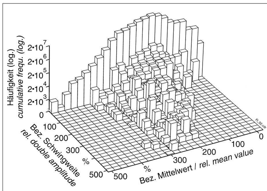
Fig. 2: Rain flow load spectra for front axle load using a front end loader, represented time: 1000 hours, based on an estimated probability of about 50% (no shock loads)
