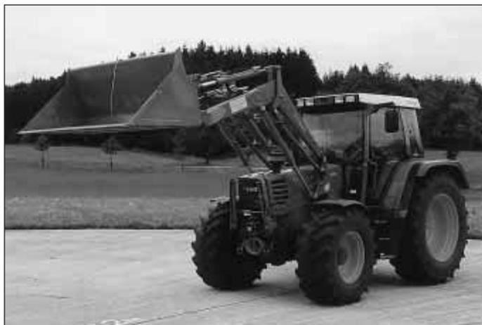
Fig. 1: Research tractor with front end loader (Fendt 509 C, 70 kW, 5400 kg, wheelbase 2328 mm)
