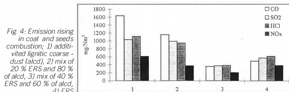
Fig. 4: Emission rising in coal and seeds combustion; 1) additivited lignitic coarse-dust (alcd), 2) mix of 20 % ERS and 80 % of alcd, 3) mix of 40 % ERS and 60 % of alcd, 4) ERS
