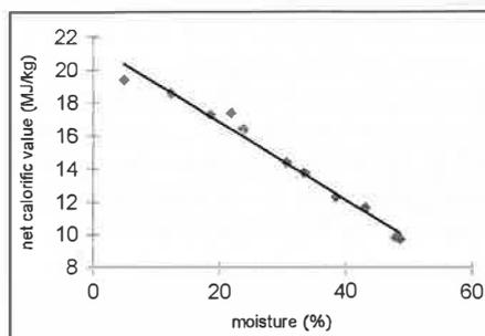
Fig. 3: Dependence on net calorific value on water contents
