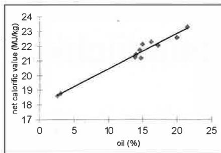
Fig. 2: Dependence on net calorific value on oil contents
