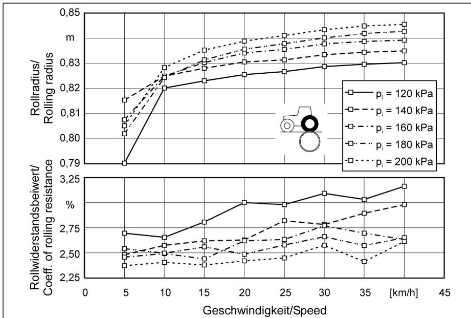
Fig.2: Coefficients of rolling resistance (at ~ 1% slip) as well rolling radii of a standard tyre Goodyear 18.4 R 38 on the roller test rig as a function of tyre pressure and speed. Static axle load: 24.6 kN
